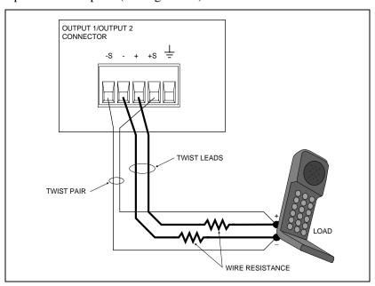
Figure 3-2. Remote Sense Connections
